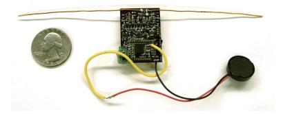
Fig. 7. The WISP with attached piezo-element.
