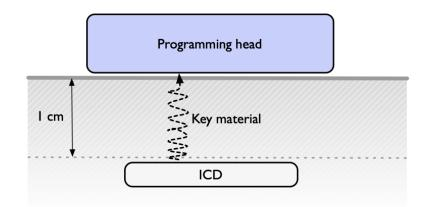
Fig. 9. Zero-power sensible key exchange: a nonce is transmitted from the ICD to the programmer using acoustic waves. It can be clearly picked up only if the programmer is in contact with the patient's body near the implantation site, and can be used as the secret key in the authentication protocol from the previous section. (1 cm is a typical implantation depth. Diagram is not to scale.)
