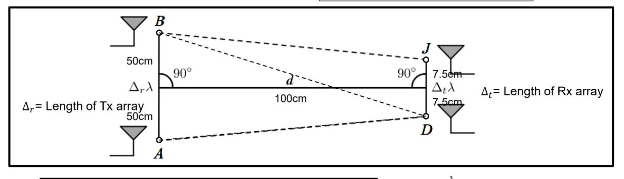
$$\delta = \overline{DB} - \overline{DA} = \sqrt{(50 + 7.5)^2 + 100^2} - \sqrt{(50 - 7.5)^2 + 100^2} = 6.7 cm(\sim \frac{\lambda}{10})$$
