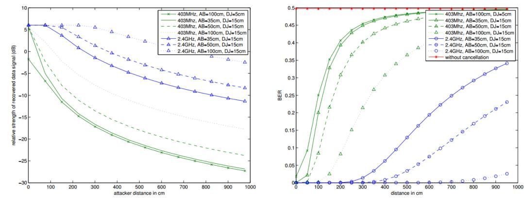
Theoretical limits for relative strength of recovered data signal
