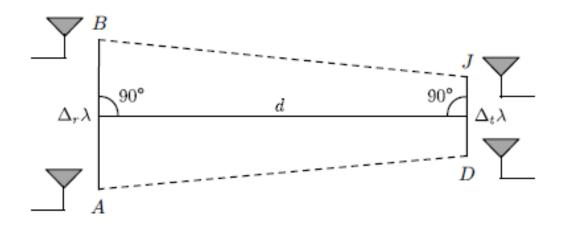
• Reduce the distance between device (D) and jammer (J).  $(\overline{DJ} \ll \frac{\lambda}{2})$ • Use multiple jammers.
