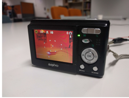
Fig. 19. Infrared viewer viewing a light-emitting infrared laser module.
