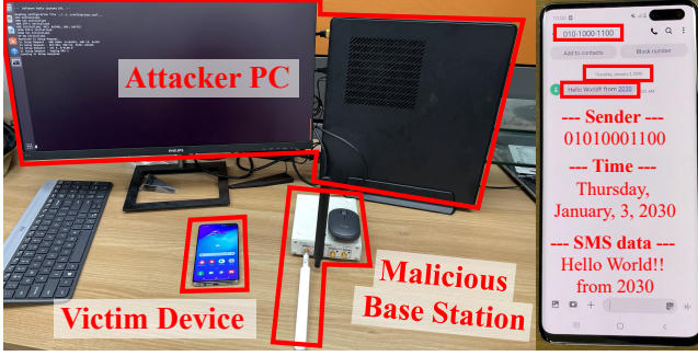
Figure 10: Exploit environment (left side) to demonstrate the NAS AKA bypass vulnerability (E4), delivering an arbitrary SMS message (right side).
