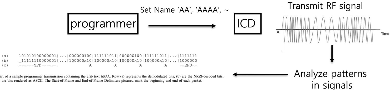
Fig. 5. Part of a sample programmer transmission containing the crib text AAAA. Row (a) represents the demodulated bits, (b) are the NRZI-decoded bits, and (c) are the bits rendered as ASCII. The Start-of-Frame and End-of-Frame Delimiters pictured mark the beginning and end of each packet.
