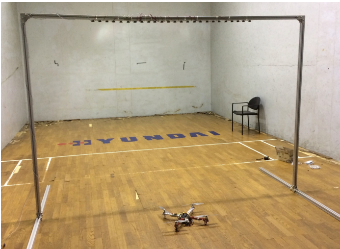
Simple sonic wall (3m-by-2m, 25 speakers)
