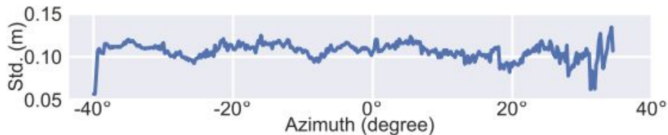
Standard deviations of inner-frame error on VLP-16
