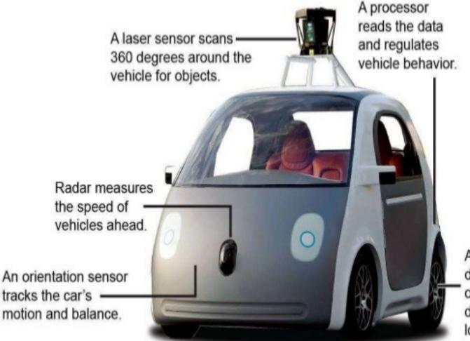
A wheel-hub sensor detects the number of rotations to help determine the car's location.
