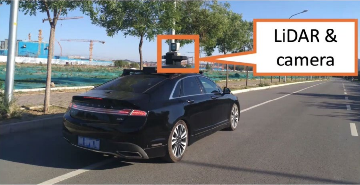
Road & car with LiDAR & camera
