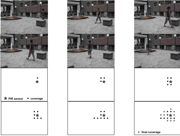
Fig. 11. Mapping Event Detection to the Event Position Using Image Capture at Time t = 6, 8, 10, 16, 17, 20 (sec); last map includes Additional Training Results by t = 40 (sec)
